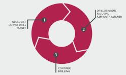
Azimuth Aligner Wireless eliminates 3 steps associated with the process of aligning a drill rig. Downtime waiting for land surveyors and geologists to approve the drill setup is removed. The rig setup can be checked by verifying the data from the Azimuth Aligner Wireless database. Bit on bottom time increases.
